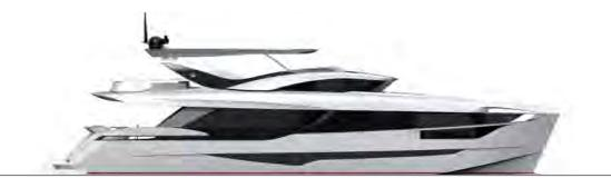
Length overall (incl. beach platform) Waterline length Maximum beam Draft 27.35 m (hull length: 23,95 m) 23.50 m 6,58 m 1.30 m (without propellers) 1.72 m (with propellers - Fortjes version) 1.85 m (with propellers - shaft version)
